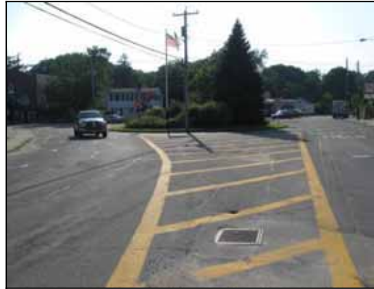
Sheet flow from upgradient private property (left) can flow into drains in public roads (right).
