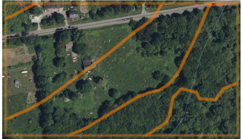
Area of Soil Map Units from the USDA NRCS Web Soil Survey
