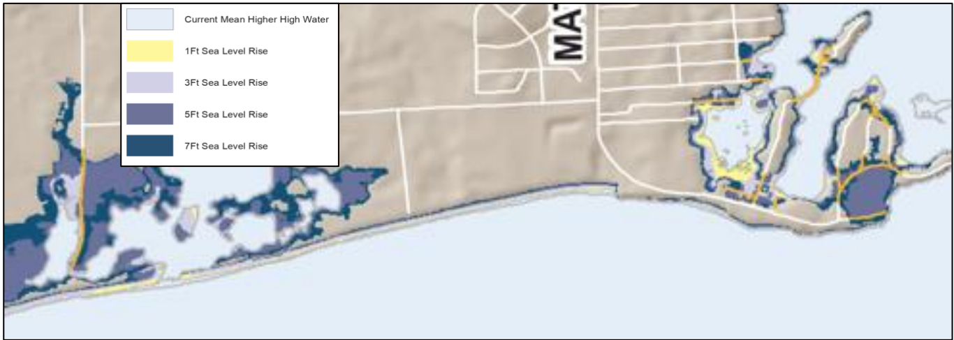
Figure 43. Sea Level Rise Scenarios Affecting Roads (Town of South Kingstown, Sea Level Rise Scenarios Affecting Roads, 2016).
