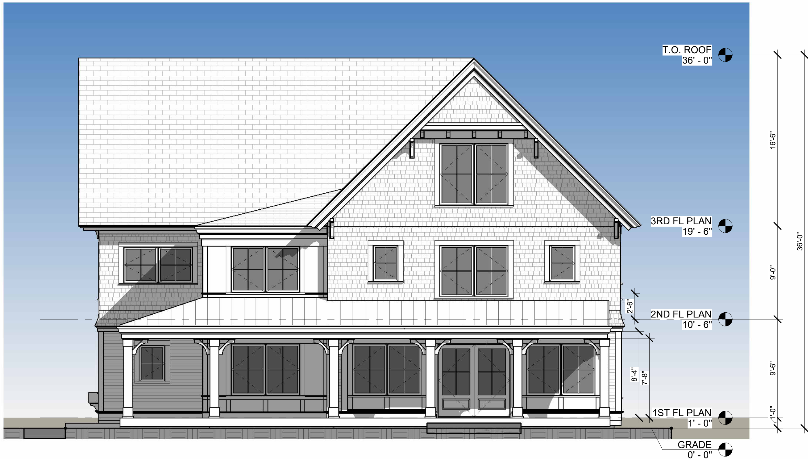
① NORTH ELEVATION - PROPOSED 3/16" = 1'-0"
