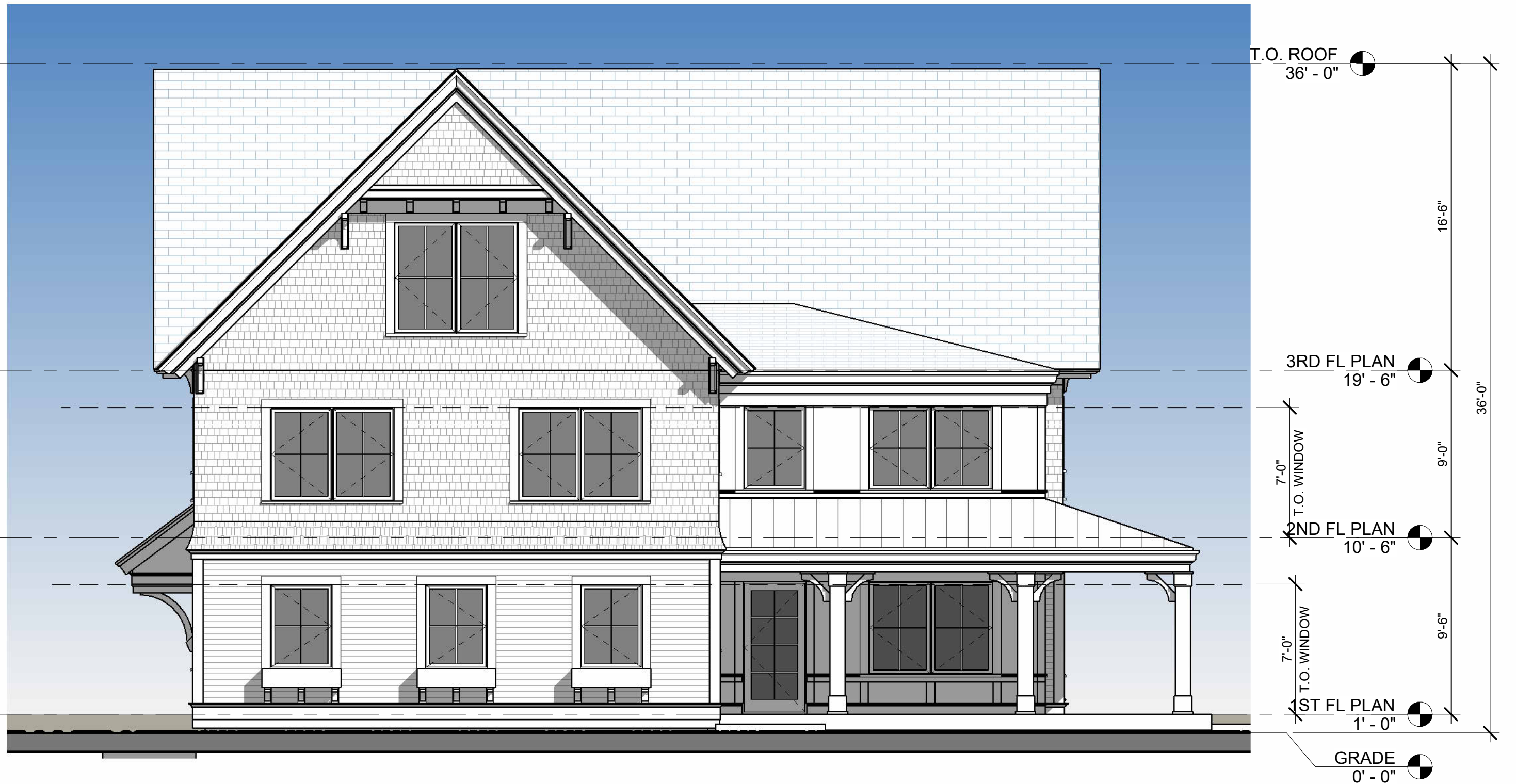
① EAST ELEVATION - PROPOSED 3/16" = 1'-0"
