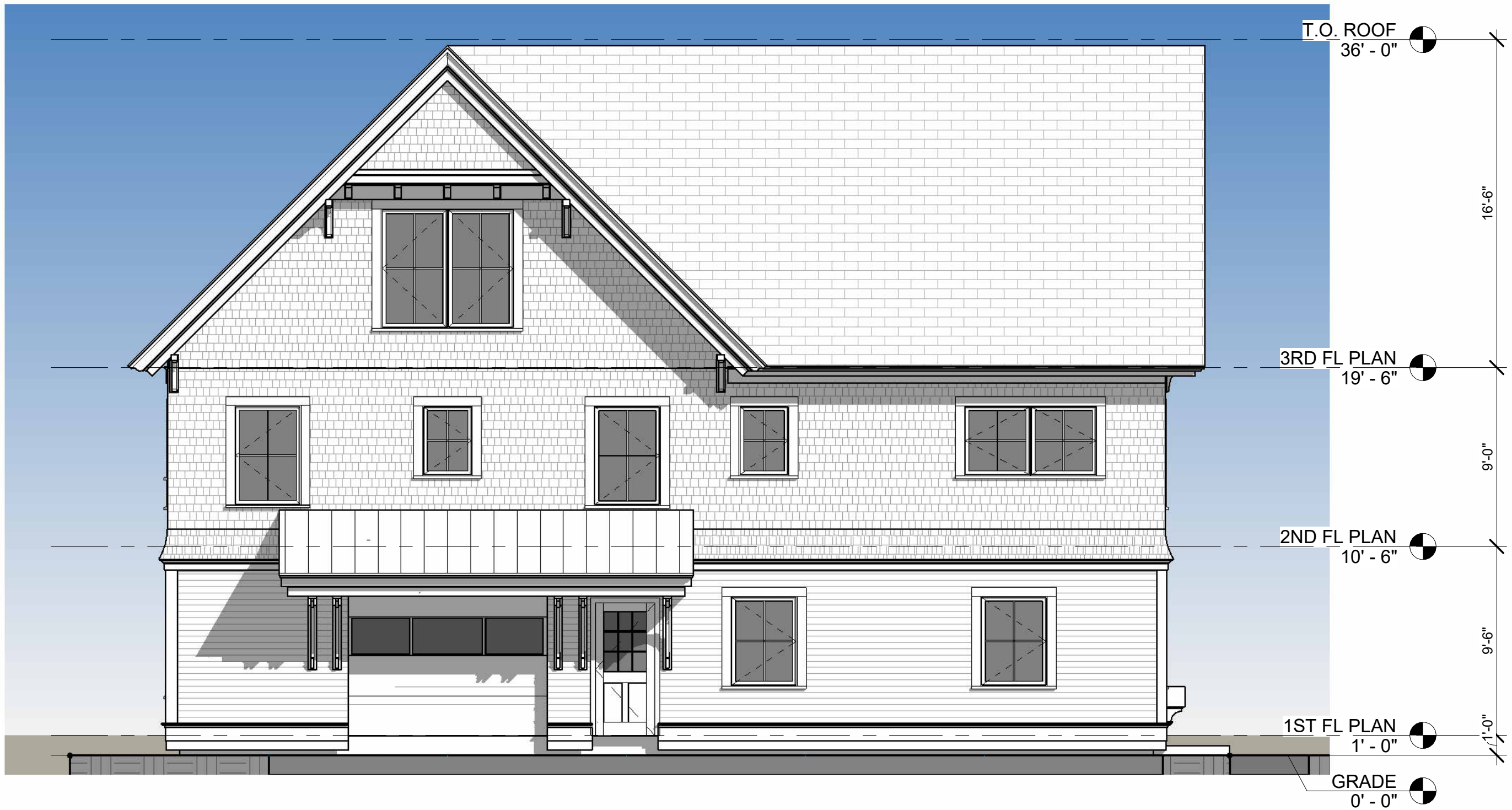
① SOUTH ELEVATION - PROPOSED 3/16" = 1'-0"
