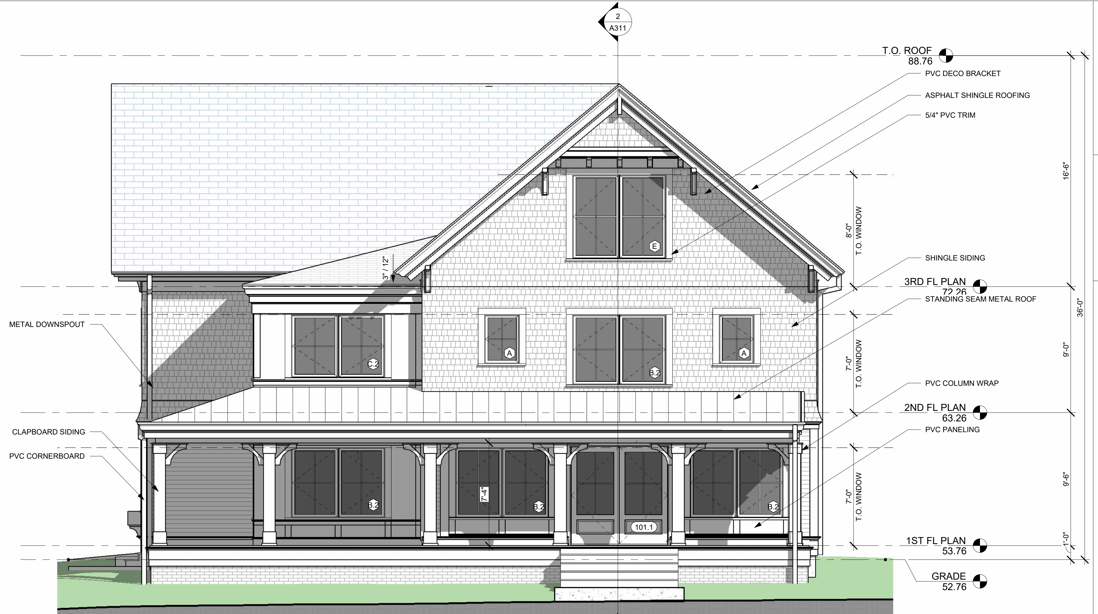
1 NORTH ELEVATION - PROPOSED 1/4" = 1'-0"
