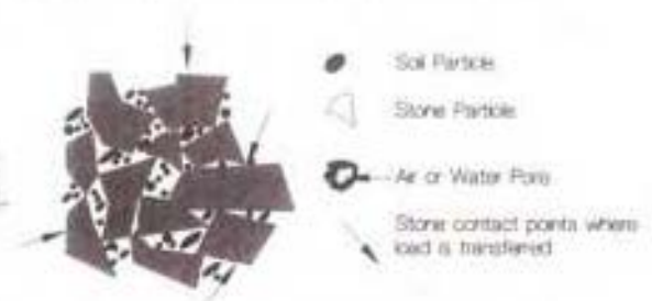
Fig. 1: The stone lattice bears loading while the soil particle partially fills the lattice voids.
